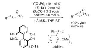
**Essential extras**: A combination of  $Y(O-iPr)_3$ , biphenyldiol ligand **1a**, and an achiral phosphorus additive enables the catalytic asymmetric epoxidation of  $\alpha,\beta$ -unsaturated phosphane oxides
