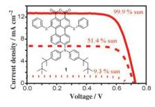
Sunny side up: 1,6-Dithiophenol-substituted perylene organic sensitizer 1 was synthesized, and its photovoltaic properties in dye-sensitized solar cells were assessed. When anchored onto TiO<sub>2</sub> film, the dye exhibits an unprecedented incident monochromatic photon-to-current conversion efficiency of 87% and yields a power conversion efficiency of 6.8% under standard AM 1.5 solar conditions.
